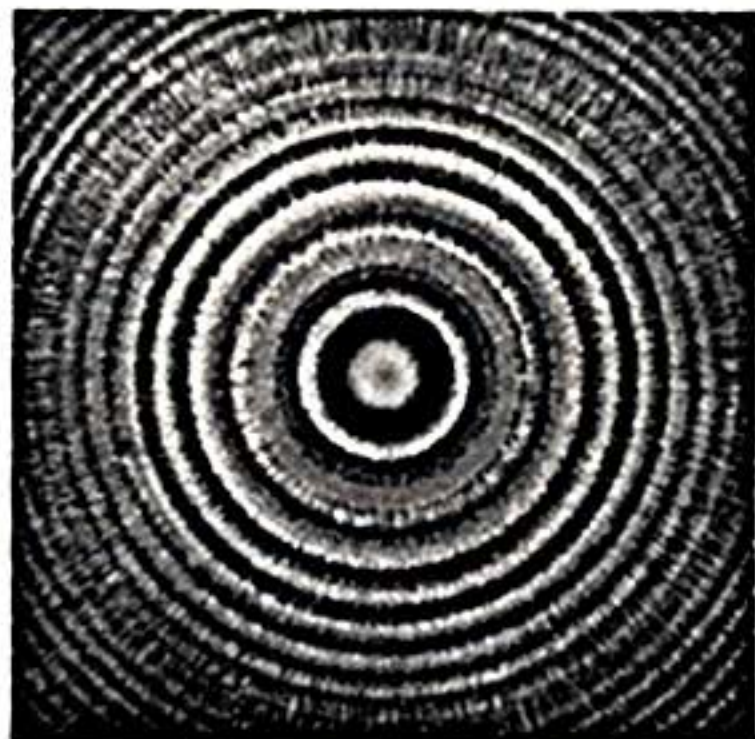
Fabry-Perot interferometer pattern in krypton-ion laser beam
